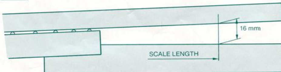
Fig. 4 SETTING NECK ANGLE (USING A STRAIGHT EDGE)
